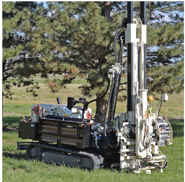
Equipment used to install sampling points
