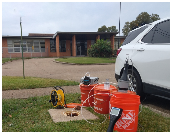
Groundwater sampling at a monitoring well
